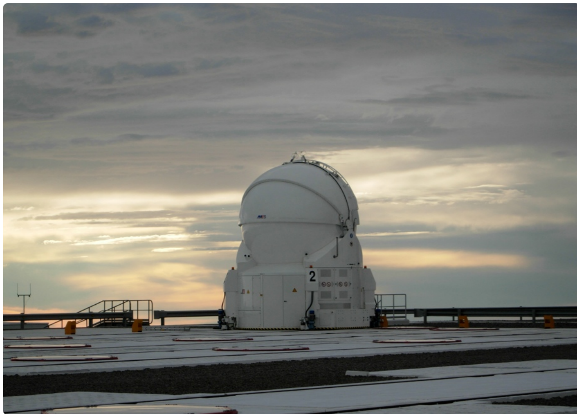
One of the 1.8m diameter auxiliary telescopes, mobile on tracks, working in synchronization with the large telescopes. Paranal, Chile, August 12, 2007. Photo: Gerhard Schmitt.
