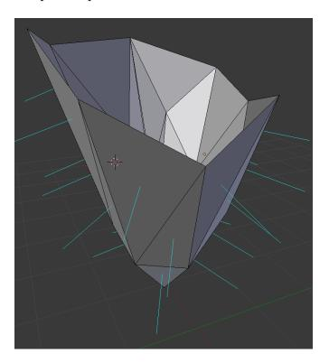
e) When you now project the points back into a plain (set scaling in z-direction to zero) and change the viewport shading to wireframe, you can see the delaunay triangulation we just constructed.
