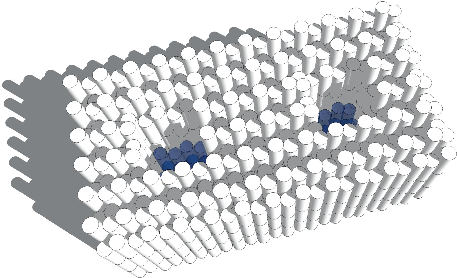
The basic element is rotated and fitted together just like bricks in a wall.
